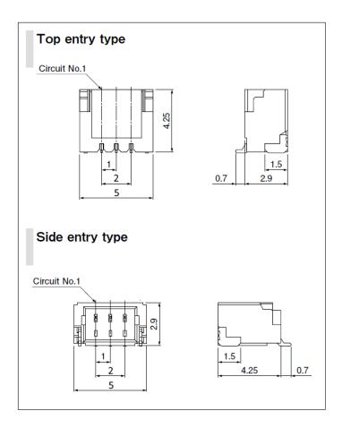
The following PCB footprints show the pin numbering for both top and side entry types and signal direction from the target perspective. For clarity, the fact that we are showing UART on a side entry type and serial debug on the top entry type is just for example – either type can use either interface:
